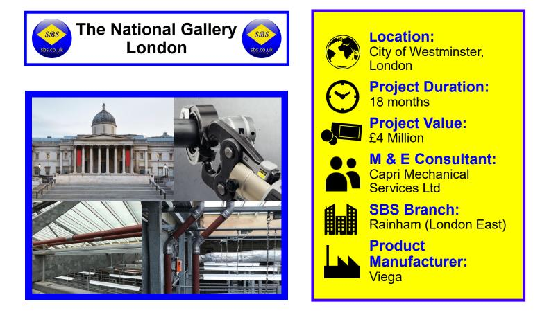
Viega's Megapress connection technology, supplied by Smith Brothers Stores, was specified as the ideal solution for a section of pipe relocation work at The National Gallery in London. The industry-first press connection system for thick-walled steel tube, Megapress, ensured that the installation of steel pipework for the building's heating and chilled water HVAC systems could take place without disruption to the gallery space which remained open throughout the project.
