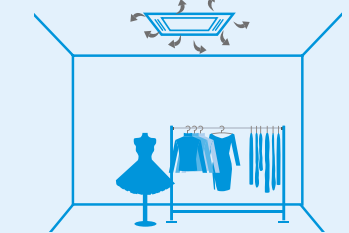
Air distribution with a dusty filter
